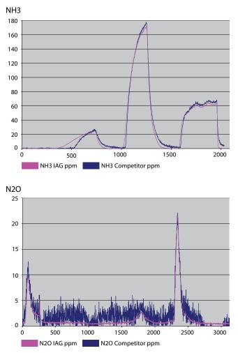
Fast response in NH 3 measurement. Clear N2O signal down to far below 1 ppm. This data was recorded in a comparative measurement with a reference system. Both samples were taken from one sample point with a flow of 7l/Min.
