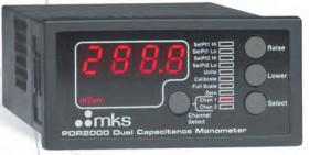
**Power Supply & Readout** — MKS offers a versatile, CE marked, low cost solution for providing power and displaying pressure output values for the MKS Baratron<sup>®</sup> family of transducers. Up to two manometers may be operated from a single PDR2000. Readings are displayed on the front panel and are also available on demand via RS232 interface. Engineering units include Torr/mTorr or mBar/microBar.
