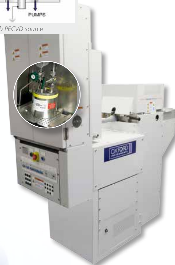
Inside view of precursor pot for liquid/solid precursors. Example: \text{Mo}(\text{CO})_6 , \text{W}(\text{CO})_6 , DMDS, DESe, DETe etc.
