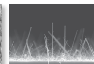
Si nanowires using Au NP as catalyst
