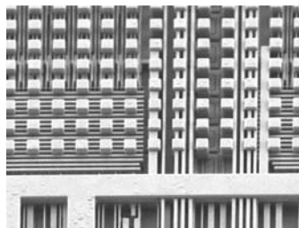
Failure analysis - fast metal layer exposure in the PlasmaPro FA ICP
