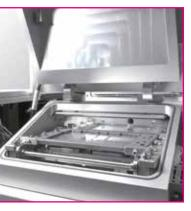
With its vacuum supported soldering process the VADU 100 system stands for high-quality void-free soldering results, even in small series production.
