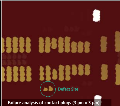
Failure analysis of contact plugs (3 \mu\text{m} x 3 \mu\text{m} )
