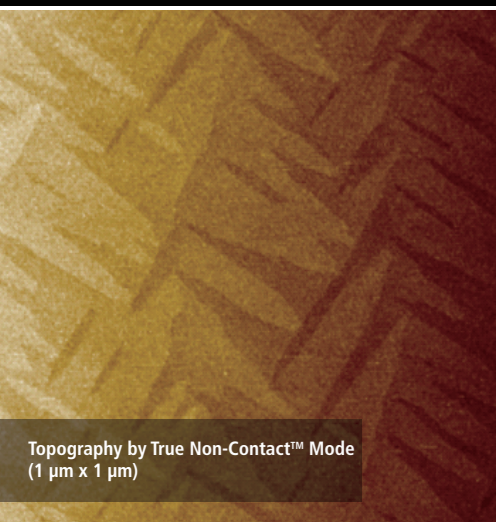
R_a = 0.94 \text{ \AA} , R_q = 1.18 \text{ \AA} True Non-Contact™ Mode (1 μm x 1 μm)
