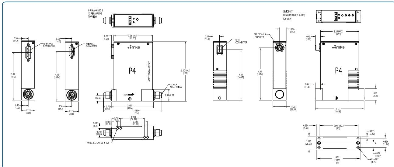
Dimensional Drawing — Analog 9 Pin D, 15-Pin D, RS-485 and DeviceNet™
