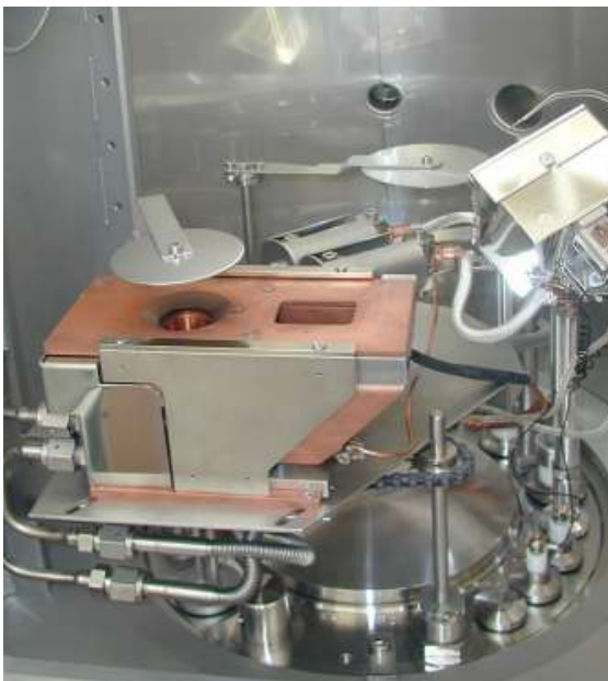
Electron beam source, two resistance sources and quartz lamp substrate heater.
