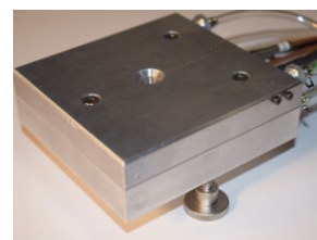
The iNano sample heating option is used to characterize mechanical properties at elevated temperatures
