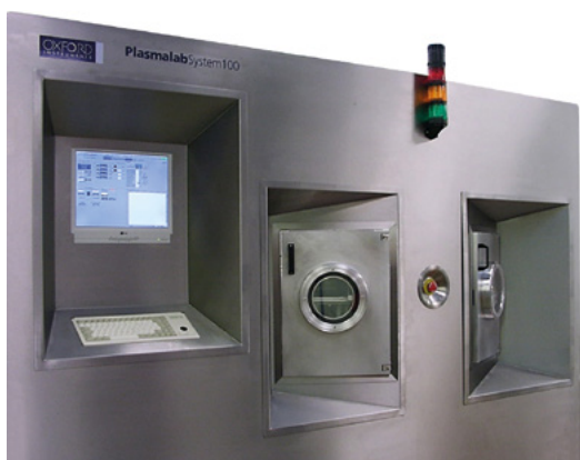
Configurations can be located entirely within the cleanroom or through-the-wall
