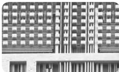
Failure analysis - fast metal layer exposure in the PlasmaPro FA ICP
