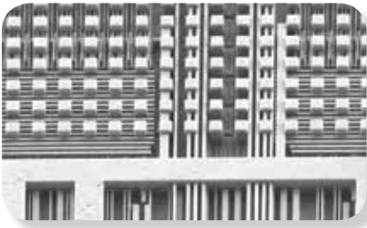
Four metal layers of a packaged device can be exposed in less than five minutes
